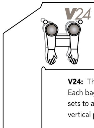
**V24:** The V24 is designed for pipe diameters up to 24". Each bag measures 84" x 96" and features two glovesleeve sets to allow easy access to all areas of a large diameter vertical pipe.
