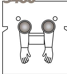
This full featured AVAIL glovebag sets the industry standard for efficiency on pipe diameters up to 10". Each chamber measures 54" x 60" with one arm set, and two ports per chamber, 6 mil construction. Available in both extended-run design on a roll or as pre-cut single bags.
