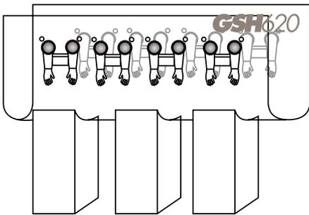
**GSH620:** Designed for large horizontal pipe, vessels, ducts and beams. 3 debris chambers/chutes channel waste away from the work area. 8 arm sets make all surfaces accessible in contained work area. Flat dimensions are 20' x 12' and can enclose work areas up to 30" in diameter. 9 mil construction.
