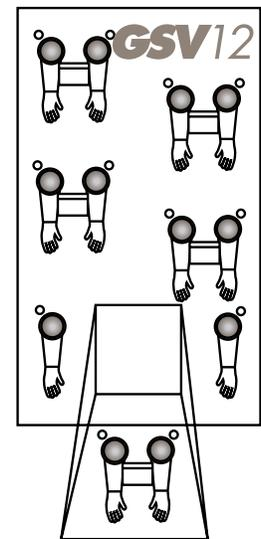
**GSV12:** This glovesheet product is designed for vertical pipes or risers up to 12' high and 12" in diameter and features a large debris chamber at the base of the sheet for waste collection. The debris area is offset from the work area, flat dimensions are 9' x 15'. 6 mil construction.
