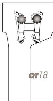
For pipe up to 18" in diameter, the QT18 model is recommended. The QT18 features two sets of glovesleeves, one on each side of the bag, to allow access all around the pipe.
