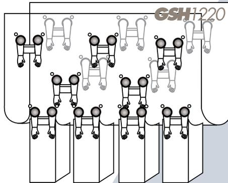
**GSH1220:** This extra large glovesheet enclosure is designed for large vessels, tanks or boilers. 14 arm sets make all areas of structures with diameters up to 72" accessible. Flat dimensions are 20' x 19' with 4 debris chambers/chutes to channel waste from the work area. 9 mil construction.
