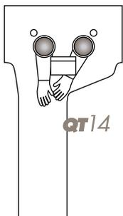
The QT14 is designed to safely enclose pipe diameters up to 14" in diameter.
