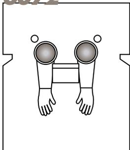
Designed for pipe diameters up to 14" in diameter. The bag measures 60" x 72" with one set of glovesleeves.
