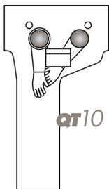
The QT10 is designed for horizontally situated pipe in diameters up to 10". The QT10 can handle up to 40% more insulation than a standard glovebag.
