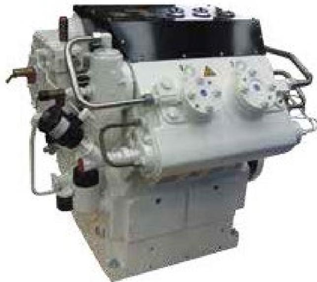
The H 5437 is a heavy duty 4 stage, water cooled, lubricated compressor set designed to operate in the harshest of environments but easy to maintain. This compressor type can manage a wide variety of gases, depending on the application. Typical gases include industrial air, breathing air, nitrogen, heliox, natural gas, helium. Other gases available. Limitations apply and subject to selection.
