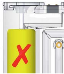
Indicator down: replace element
