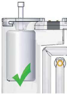
Indicator is up: element is clean
