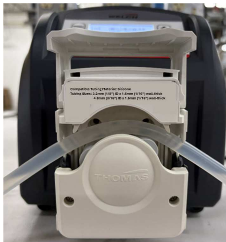
Figure 19 – shows the pump head with the tubing positioned properly before the pump head is closed.
