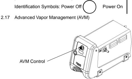
Advanced Vapor Management (AVM) is provided for precise setting of vacuum level.
