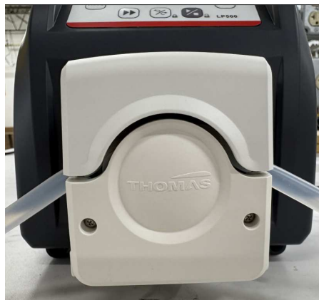
Figure 20 – shows the pump head after it is closed with the tubing installed.
