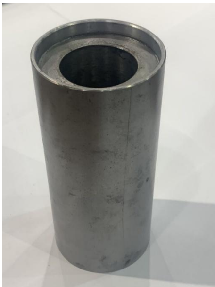
564-024 Sideplate oil seal press tool—P1057
