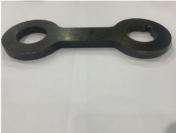
564-029 Rotor Timing Lock—P1057
