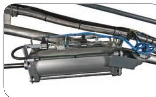
Pneumatic device to move the primary arm and hold down the cone to seal the manhole for vapor recovery.
