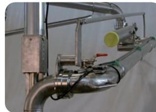
Parallel device to keep the filling tube horizontal all the time.
