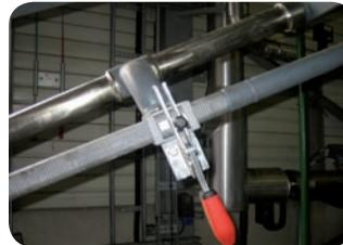
Arresting device for working position.
