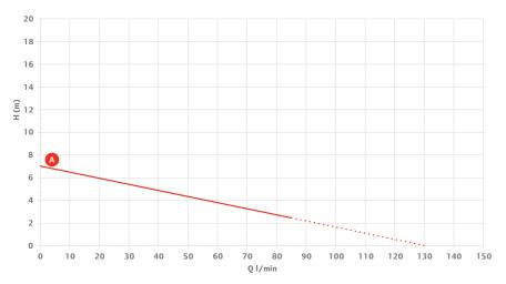
— A (Axial impeller with basic dispense kit) ..... (Axial impeller without dispense kit) Measurement under ideal conditions without pipe friction resistance. Basis: 1 mPas, 20°C, +/- 10%
