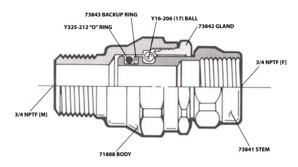
DO NOT EXCEED MAXIMUM WORKING PRESSURE OF 1000 PSI (69 BAR).
