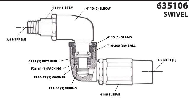
DO NOT EXCEED MAXIMUM WORKING PRESSURE OF 8,000 PSI (552 BAR).
