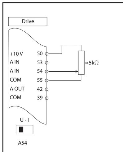
**NOTE:** Once parameter 420 is set to "[6] Analog in 54", this will be the source of the torque limit setting whether the VFD is in "Hand On" or "Auto On" mode. The pump will not operate if there is no signal on A54 or if the signal is too low.
