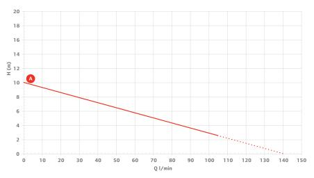
A (Axial impeller with chemistry dispense kit) ..... (Axial impeller without dispense kit)
