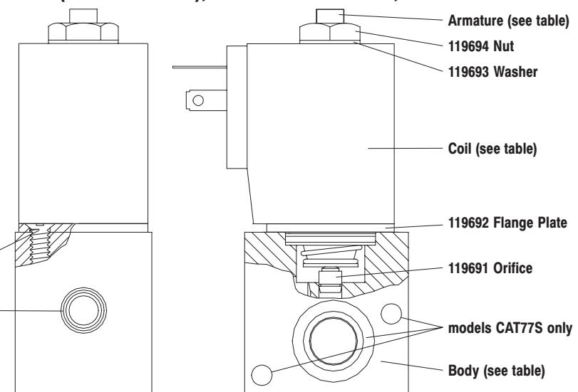
**3-WAY, NORMALLY OPEN (PASSING), 1/4 - 18 PIPE PORTS, PORTED BODY.**
