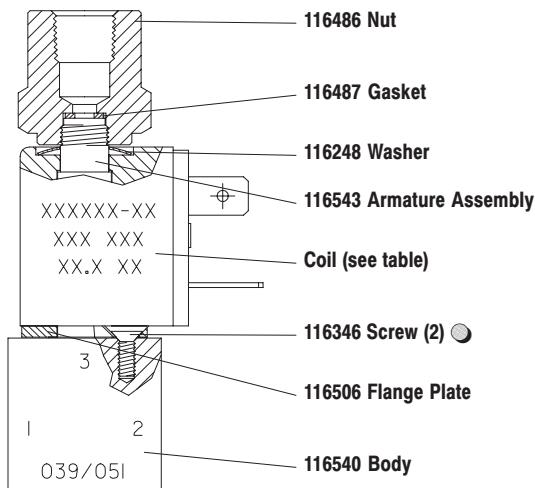
**CAT66P-( )-(): 3-WAY, NORMALLY CLOSED (NON-PASSING), 1/4 - 18 PIPE PORTS, PORTED BODY.**
