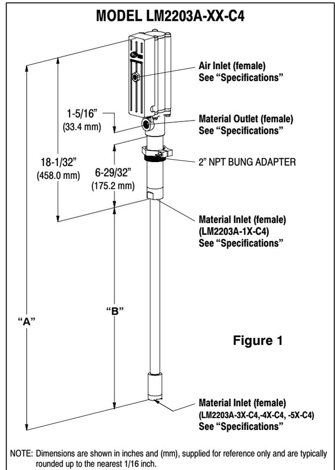
NOTE: Dimensions are shown in inches and (mm), supplied for reference only and are typically rounded up to the nearest 1/16 inch.
