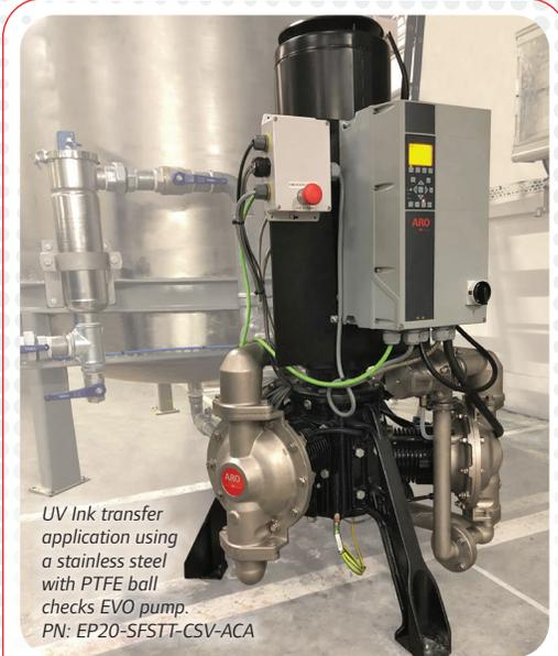
UV Ink transfer application using a stainless steel with PTFE ball checks EVO pump.
