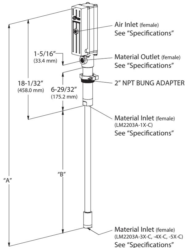
**NOTE:** Dimensions are shown in inches and (mm), supplied for reference only and are typically rounded up to the nearest 1/16 inch.
