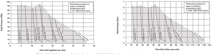
E2P10-XXXXX-CX-XXA Maximum Outlet Working Pressure 190 PSIG (13.1 bar). End user piping design must be rated to withstand this pressure.
