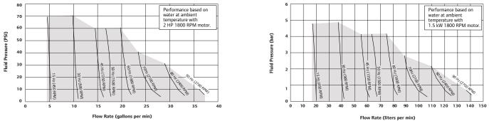
E2P10-XXXXX-BX-XXA Maximum Outlet Working Pressure 140 PSIG (9.65 bar). End user piping design must be rated to withstand this pressure
