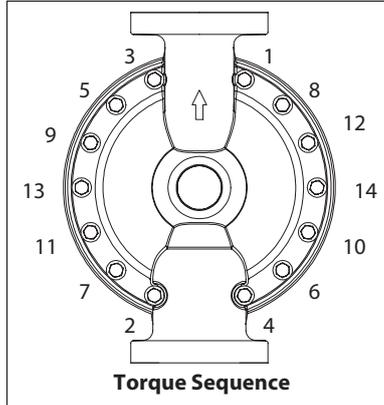
View for PW20P-YXS-XXI (PTFE diaphragm)/ PW20P-YXS-XXL (Long Life PTFE diaphragm) configuration only.
