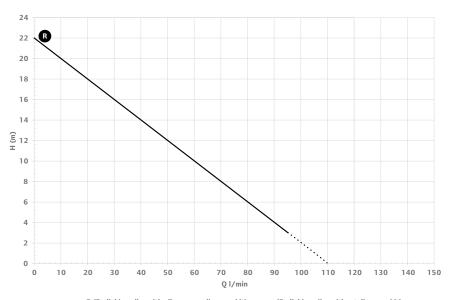
R (Radial impeller with all-purpose dispense kit) ..... (Radial impeller without dispense kit)
