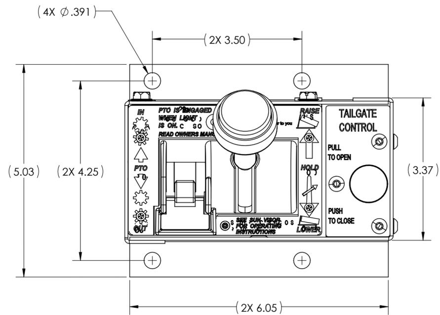
1. HOIST CONTROL (AIR) W/CONTROLLED LOWER.
