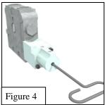
Once assembly has been completed, <u>APPLY THREAD</u> <u>SEALANT TO ALL FITTINGS</u>, install fittings and airlines and test for proper operation.
