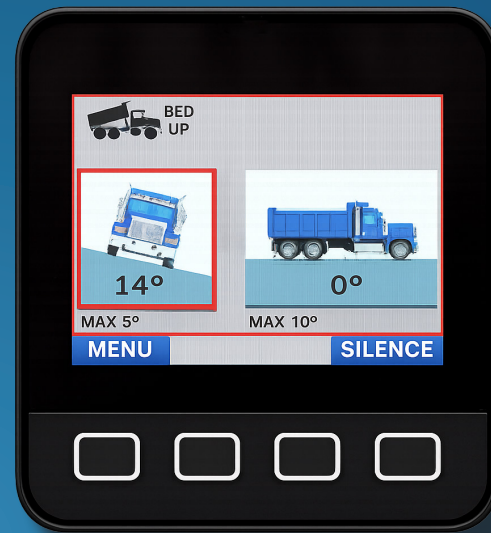
UNSAFE GROUND WARNING
