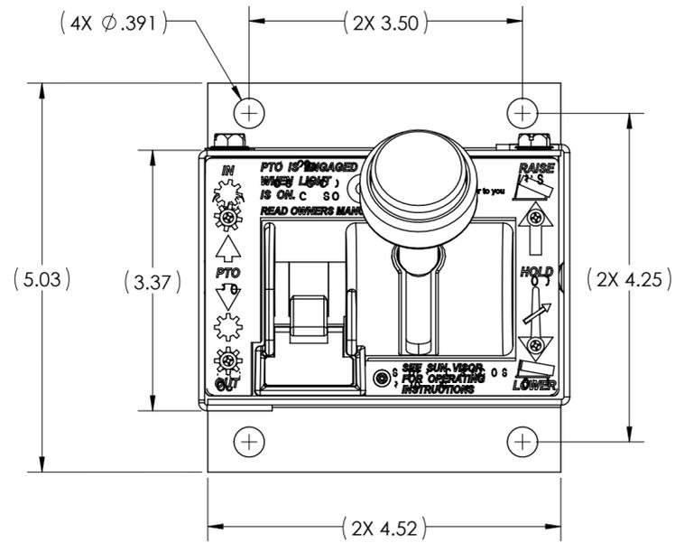
1. HOIST CONTROL (AIR) W/CONTROLLED LOWER.
