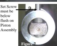
8. Grease O-Rings and slide Cylinder Body over Piston Assembly as shown in Figure 7.
