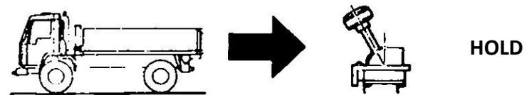
When UNLOADED leave the cab control in “HOLD” to minimize body bounce.
