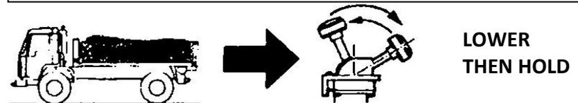
When LOADING, put the cab control in “LOWER” to insure that no oil is trapped in the cylinder and the entire load rests on the chassis. Return the control to “HOLD” when traveling.
