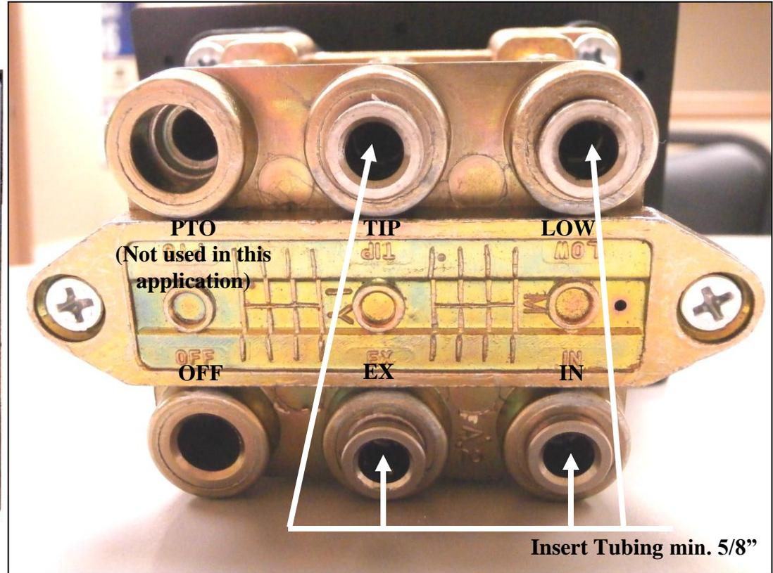
Insert tubes a minimum 5/8'' into all ports.
