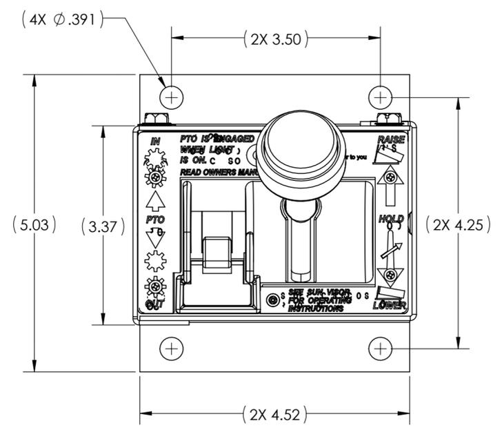
1. HOIST CONTROL (AIR) W/CONTROLLED LOWER.
