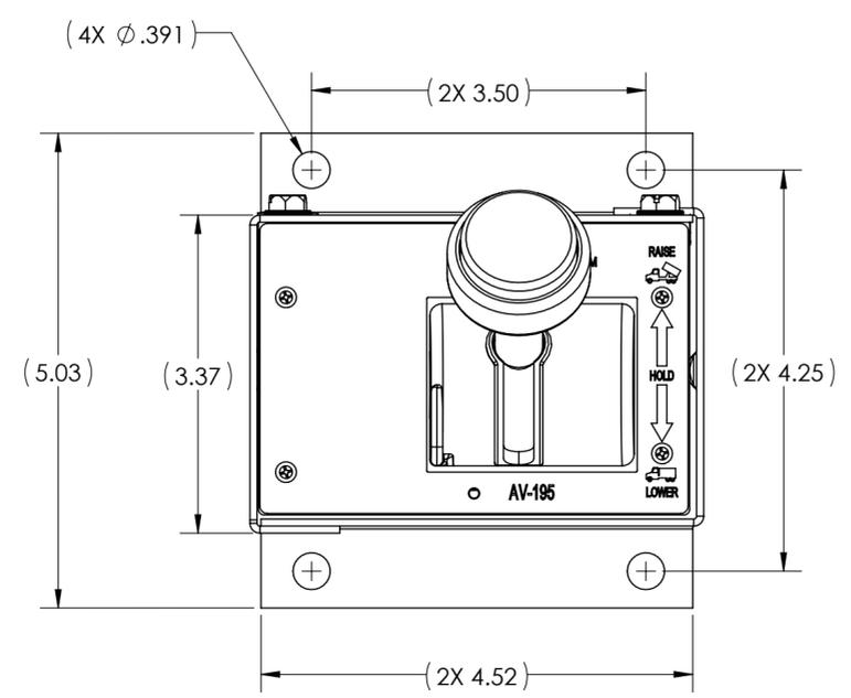
1. HOIST CONTROL (AIR) W/CONTROLLED LOWER.
