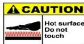
**Caution:** Surface May be Hot. Ensure PTO is off and unit has cooled before servicing.
