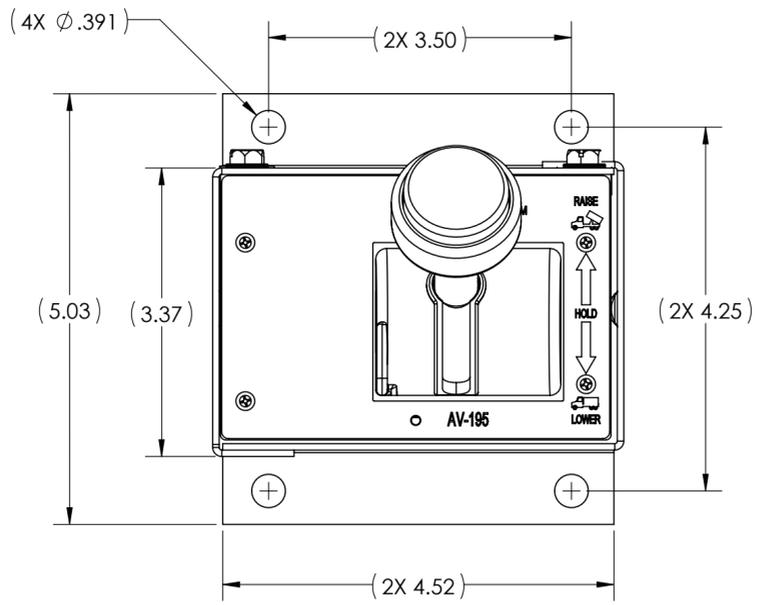
1. HOIST CONTROL (AIR) W/CONTROLLED LOWER.
