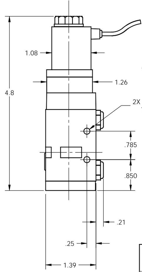
2X 1/8"-27 NPT EXHAUST PORTS W/ SINTERED BRONZE MUFFLERS
