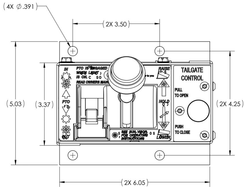
1. HOIST CONTROL (AIR) W/CONTROLLED LOWER.
