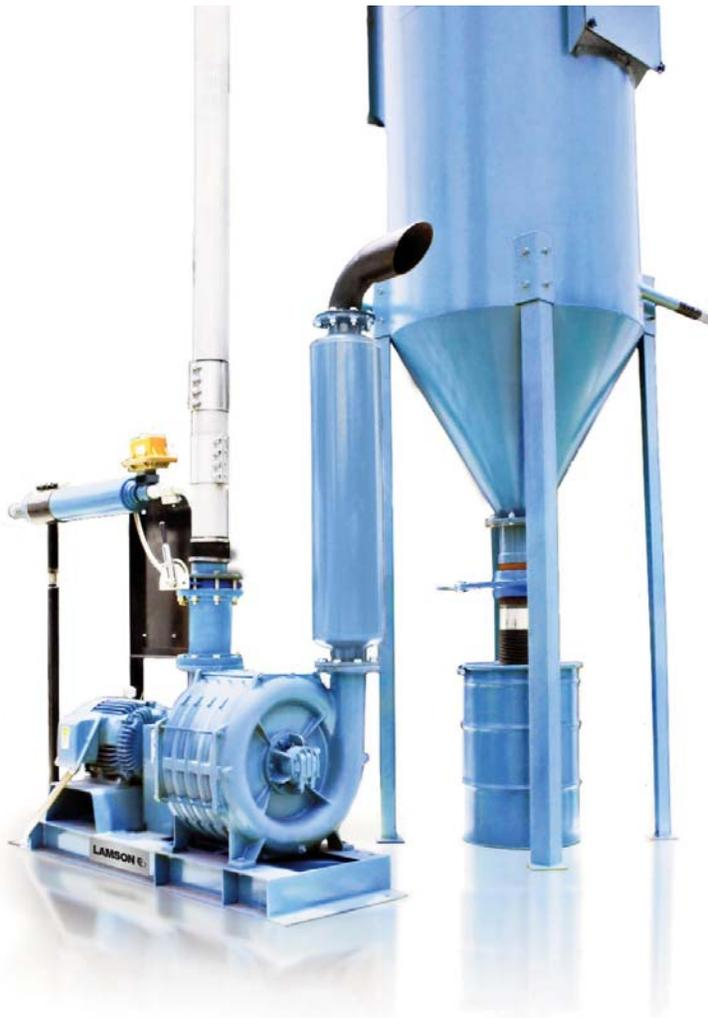
Central vacuum systems differ from traditional pneumatic conveying systems or dust collection systems. Pneumatic conveying systems have a defined source and destination while a central vacuum system varies in the number and location of the pick-up vacuum points. Most systems are designed for multiple users and thus they need to perform equally well when one or multiple users are using the system at one time.
