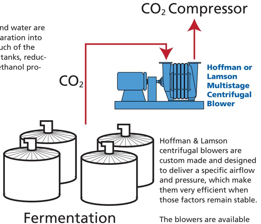
Hoffman & Lamson centrifugal blowers are custom made and designed to deliver a specific airflow and pressure, which make them very efficient when those factors remain stable.
