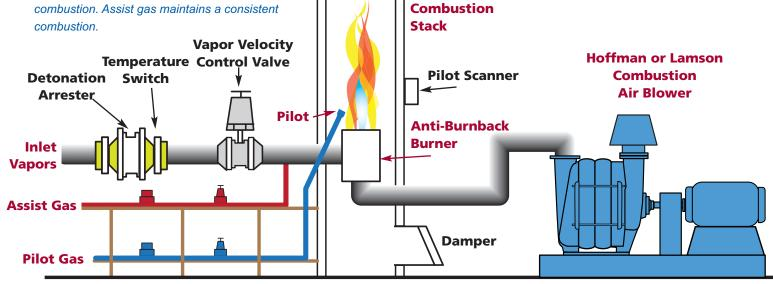
Thorough mixing is necessary to ensure that all waste and fuel come in contact with oxygen. Because complete mixing generally is not achieved, excess air/oxygen is added (above stoichiometric or theoretical amount) to ensure complete combustion.
