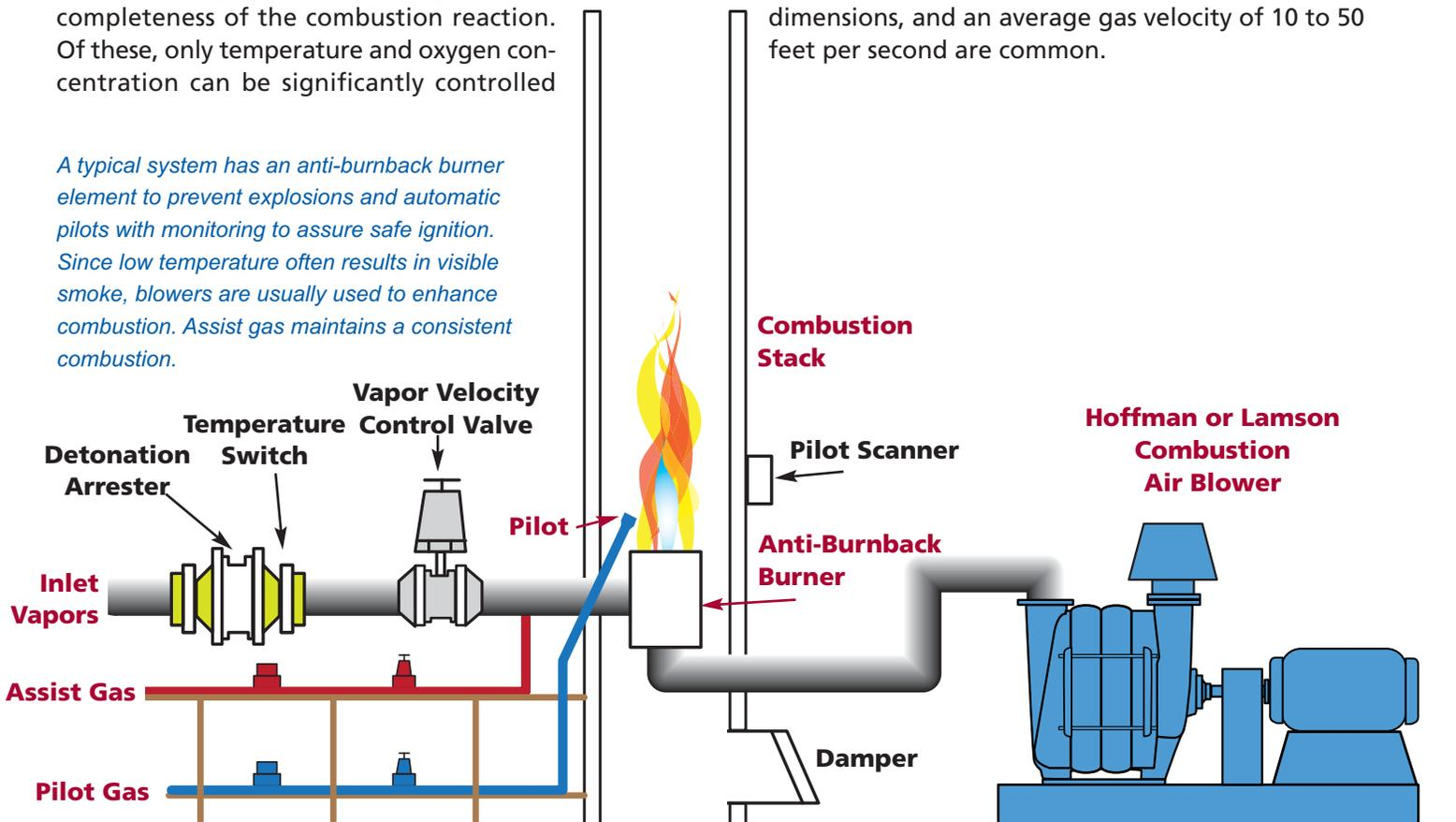
Thorough mixing is necessary to ensure that all waste and fuel come in contact with oxygen. Because complete mixing generally is not achieved, excess air/oxygen is added (above stoichiometric or theoretical amount) to ensure complete combustion.
