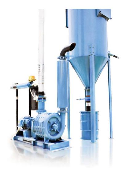
Central vacuum systems differ from traditional pneumatic conveying systems or dust collection systems. Pneumatic conveying systems have a defined source and destination while a central vacuum system varies in the number and location of the pick-up vacuum points. Most systems are designed for multiple users and thus they need to perform equally well when one or multiple users are using the system at one time.
