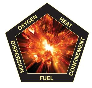
If a dust cloud is ignited within a confined or semi-confined area, it burns very rapidly and may explode. This initial explosion may shake loose more dust or damage a dust containment system. As a result, the additional dust may cause secondary explosions which can be far more destructive than the first one due to the increased quantity and concentration of the dispersed combustible dust.
