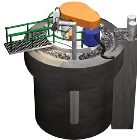
The minerals that do not float into the froth are referred to as the flotation tailings or flotation tails. These tailings may also be subjected to further stages of flotation to recover the valuable particles that did not float the first time. The final tailings are normally disposed of as mine fill or sent to tailings disposal facilities for long-term storage.
