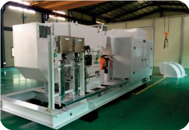
*ETO System with Junction Boxes, Skid Wiring & Sound Suppression*
