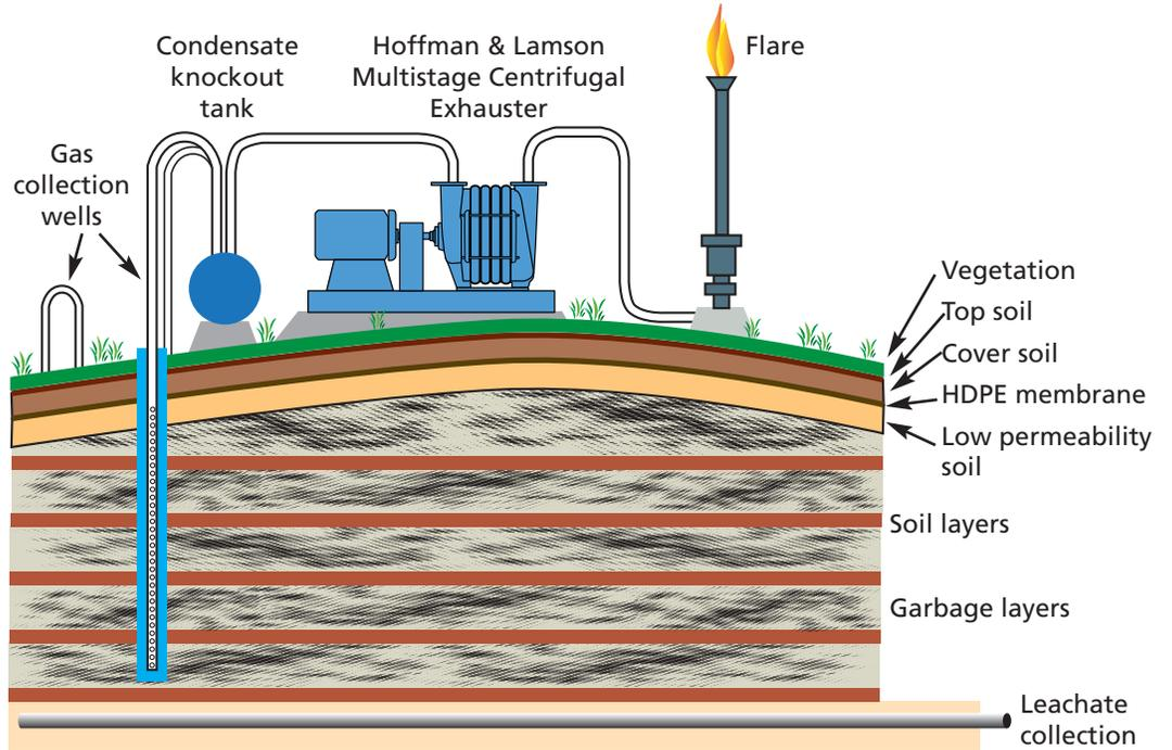
This process can use one or multiple exhausters. A single exhauster could draw from twenty to fifty pipes, however the vent pipes must be engineered to draw an even vacuum. Using multiple exhausters makes this less of a problem.
