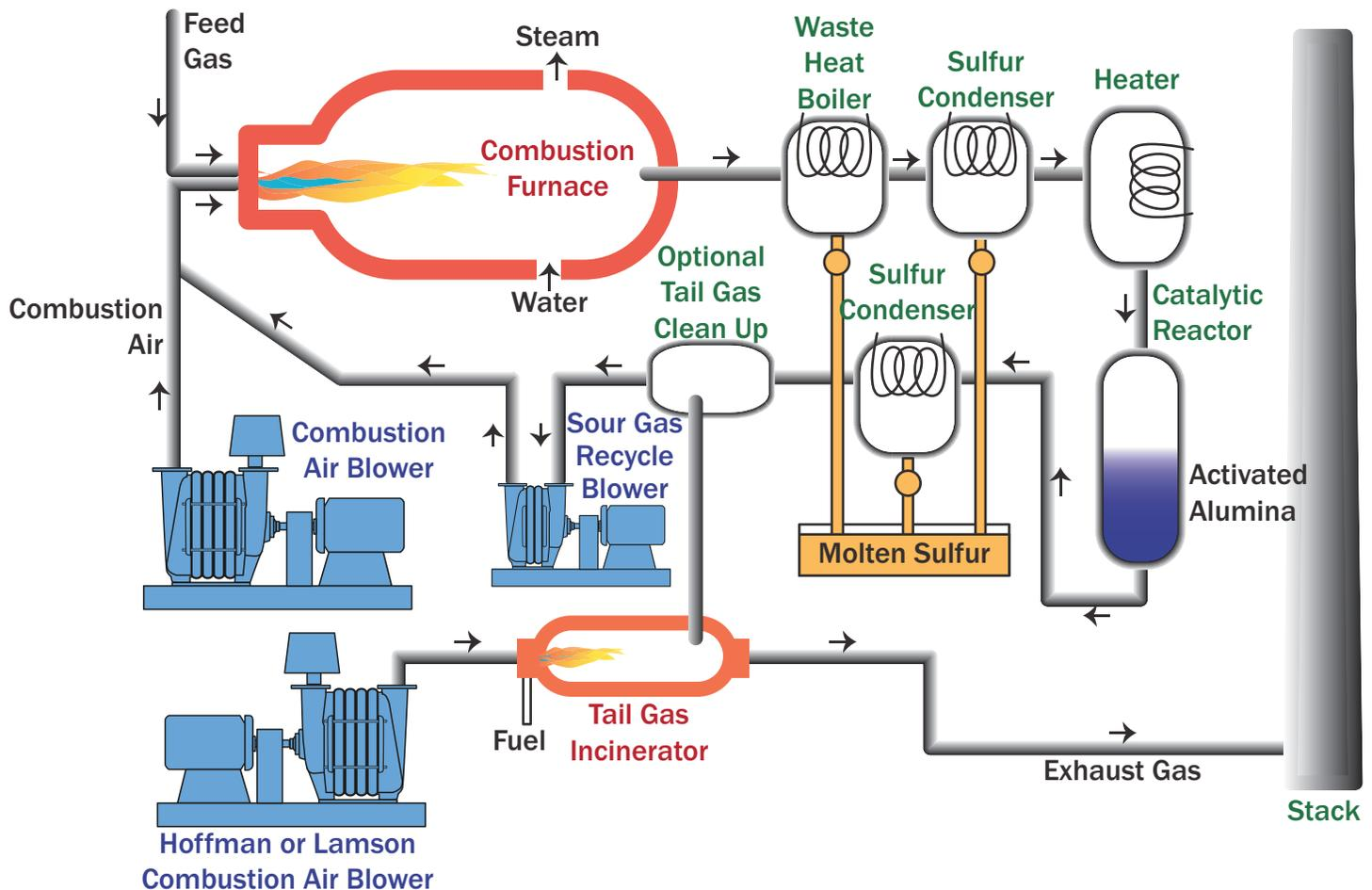
The hot reaction product gas, containing gaseous sulfur, is used to produce steam in a boiler (called a waste heat boiler) which serves to cool the gas. It is further cooled and condensed in heat exchangers while producing additional steam. The condensed liquid sulfur is separated from the remaining unreacted gas in the condenser and sent to product storage.
