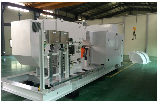
ETO System with junction boxes, skid wiring & sound suppression
