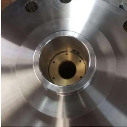
10. Use pliers to hold hardware (screw and lock washer) and place a small amount of Loctite on end of screw. Place screws into internal holes and install them down with Allen key.
