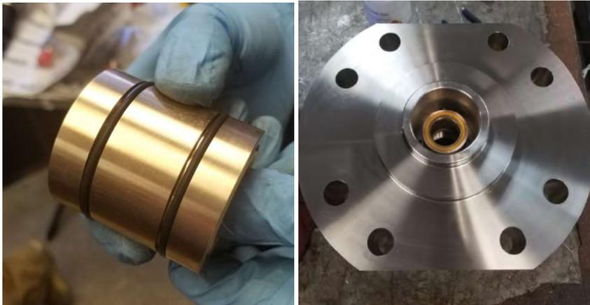
8. Use hammer and tool to install the Adapter Piece Insert so it is flush with internal surface (shown below).
