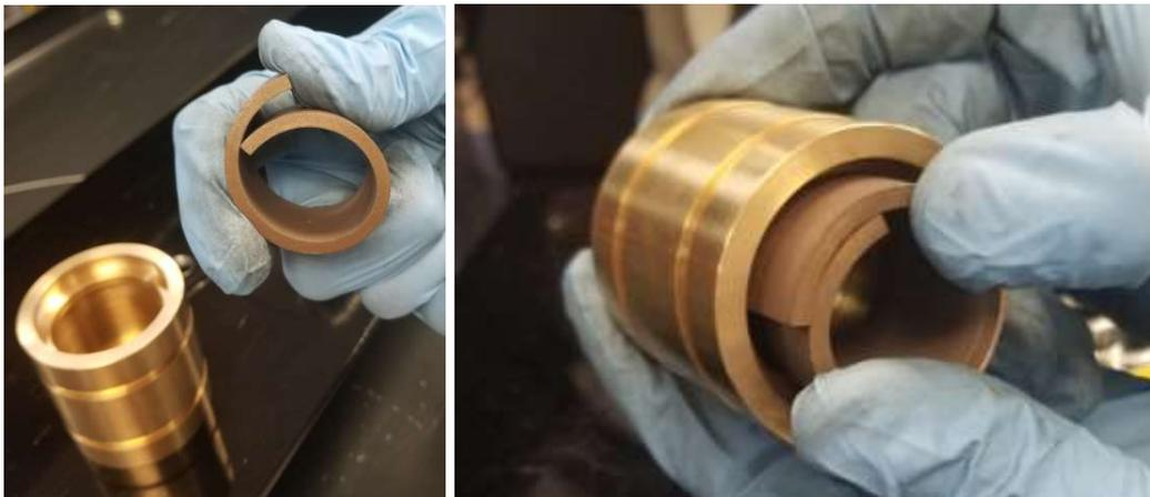
3. Install ring until edges are flush and ring is flat against internal diameter.
