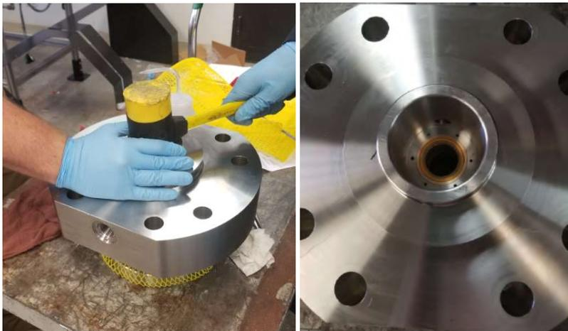
9. Install Adapter Insert Cap. Align holes with adapter plate below.
