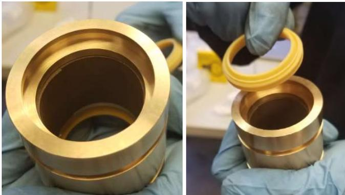
6. Wiper seal should sit flush with edge as shown below.
