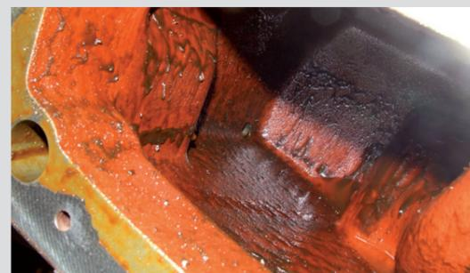
View within the gear box of a GHH RAND SILU® compressor: Surfaces heavily contaminated by congealed low-grade motor oil. Only utilization of Silol®/Silol® FG guarantees optimum lubricant lifetime and performance.
