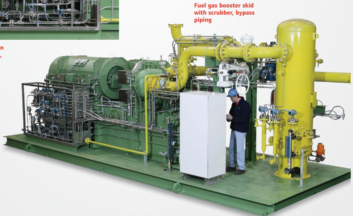
**Fuel gas booster skid with scrubber, bypass piping**
