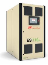
The ES Series processes cooling air within the compressor package, and a heat exchanger cools this internal air before recirculating it back. This design prevents dust and particulates from entering the compressor's interior and at the same time allows to capture even the radiation heat of internal components like motors, inverters, coolers etc. and makes this heat available for heat recovery.
