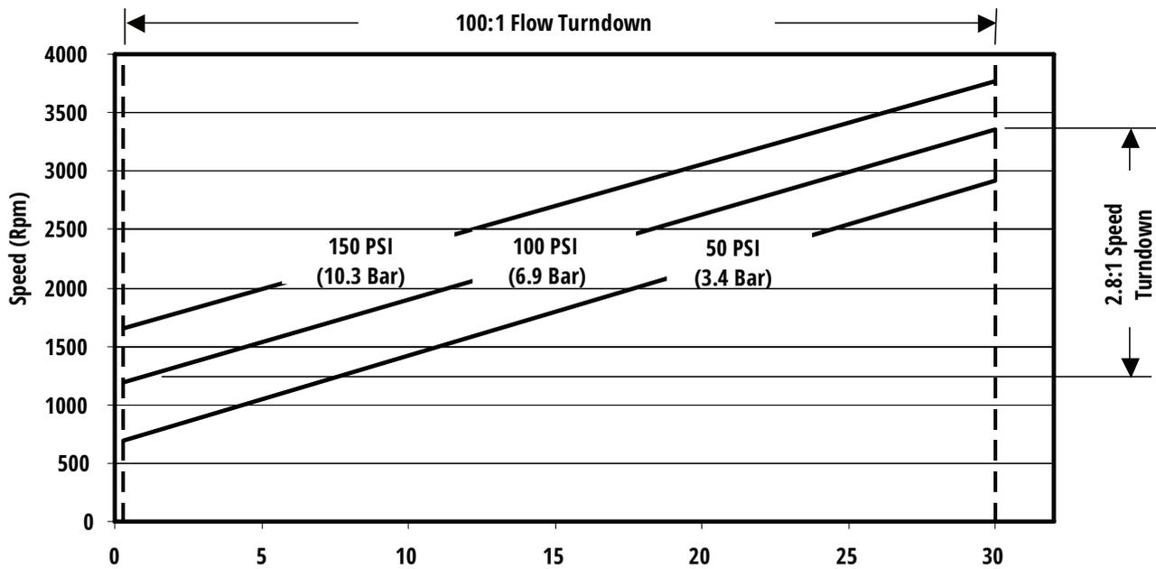
**Note:** For this application, the 0.68 ml/rev displacement pump at 100 psi (6.9Bar) differential pressure, achieves a 100:1 flow turn down with a 2.8:1 speed turn down.
