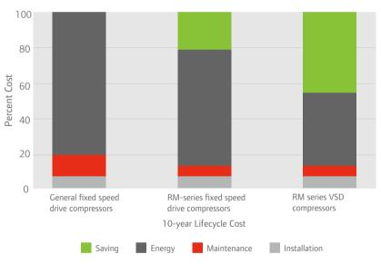
Operate at 79% load for 4,000 hours per year; 0.05\$/kWh
