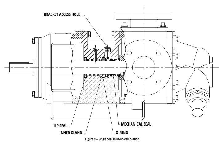
It is always recommended to replace the rotor if scoring is present on the shaft. If the old one is being re-used, lightly polish the shaft in order to remove minor defects.
