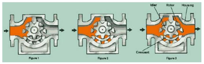
Figure 1 – Internal Gear Pumping Principle
