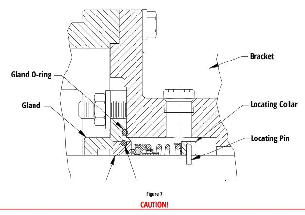
The highly polished seal faces should not be touched during the assembly process, as any minor scratch could result in leakage once in service.
