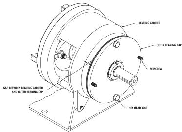
Figure 11 – Setting End Clearance
