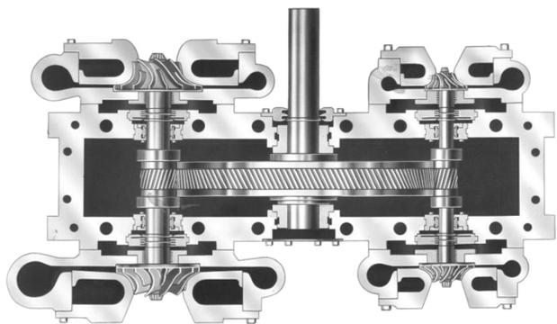
**Figure 1.** This figure shows the top view of an Ingersoll Rand MSG integrally geared centrifugal (IGC) compressor with cross-section taken at the horizontal split line of the compressor gearbox (the approximate plane at which the input shaft enters the gearbox).
