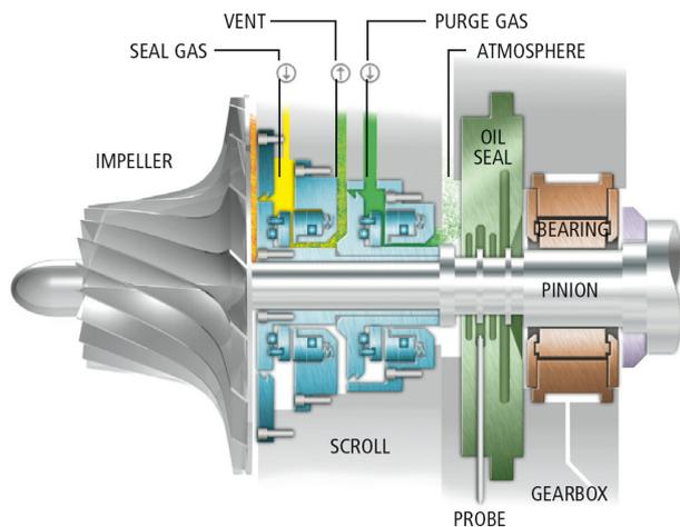
**Figure 4.** Tandem dry-face seal with integral labyrinth.
