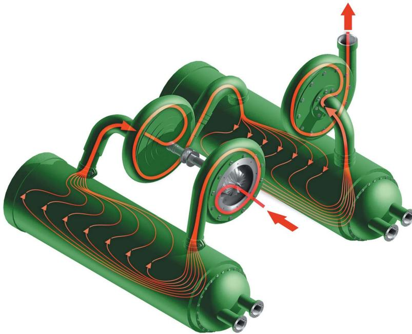
**Figure 6.** This shows the typical process gas flow path for a three-stage Ingersoll Rand MSG IGC compressor with intercoolers (the gearbox has been excluded from this illustration to provide an unobstructed view of the flow path).
