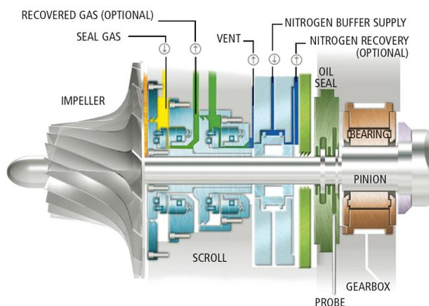
**Figure 5.** Tandem dry-face seal with carbon ring backup.
